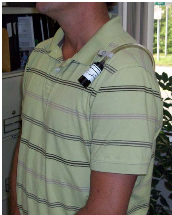
FIGURE 2: Filter cassette attached within worker's breathing zone
