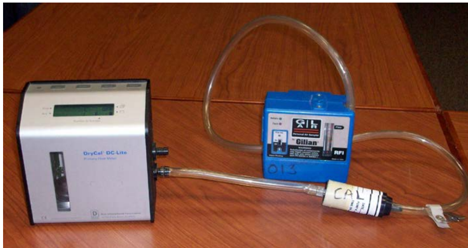
FIGURE 1: Example of sample pump connected to calibrator
