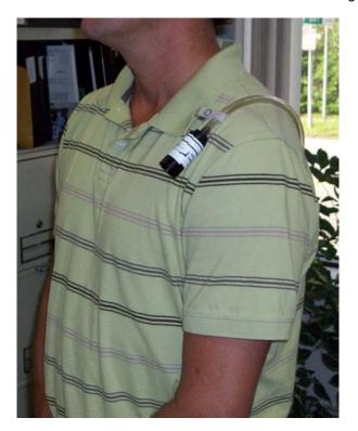
FIGURE 2: Filter cassette attached within worker's breathing zone
