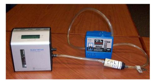
FIGURE 1: Example of sample pump connected to calibrator
